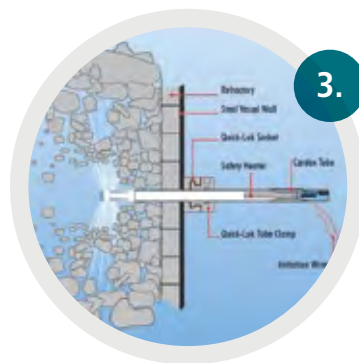
The Cardox® silo cleaning system breaks up clogged-up material in bulk containers by suddenly releasing liquid carbon dioxide
