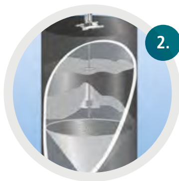
With this silo cleaning system, the hydraulically powered whips attached to a high strength, multi-part telescopic arm gently remove the deposits from the container
