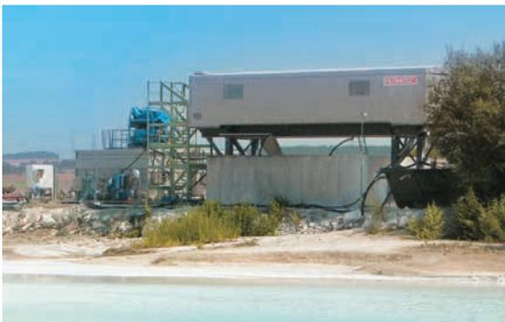
Even treating large sludge volumes is possible with mobile plants – in part we can produce up to 300 t filter cakes per shift
